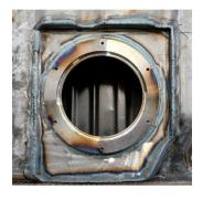
Fuel pump can now be fitted in the tank to check the height is correct, making sure that it sits flat on the bottom of the tank.
