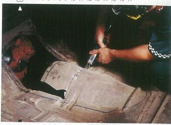
Although a factory VN/VP shifter could have been used, this installation utilised a B&M Hi-Tek Street Bandit shifter. Careful routing of the shifter's cable, with no sharp turns or tight bends, will ensure smooth operation. B&M supplies detailed fitting instructions — take note of its recommendations, as there are no short cuts
