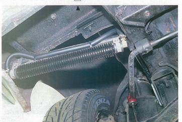
After a tweak or two to the exhaust system (for gearbox and crossmember clearance), the EK's ready to test drive. Note how the gearbox crossmember enables the handbrake to be relocated off to the side, away from its factory location (in the centre), while the tailshaft loop stops the handbrake cable from fouling the tailshaft
