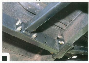
To gain adequate gearbox clearance, a section of an original floor crossmember must be removed. Do not remove this section until the three-quarter chassis kit has been installed. This ensures the unibody's construction and strength are not undermined. Note the bolt-in, round-tube tailshaft catch-bar
